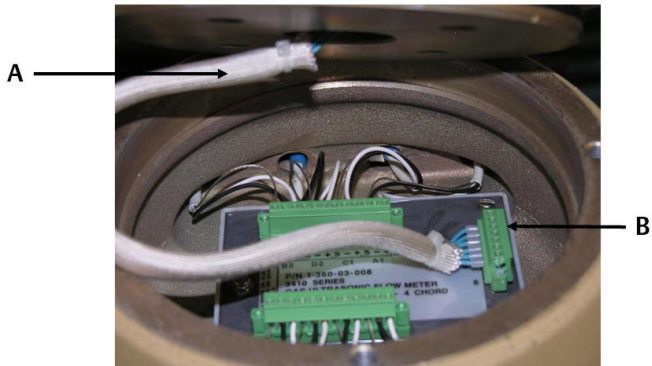
Figure 2-2: Remove Acquisition Cable and Module
