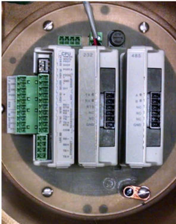
Figure C-1: 3410 Upper Electronics with Optional I/O Modules
