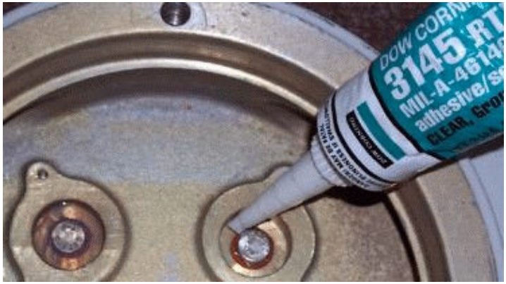
Figure 2-5: Apply RTV Sealant Around Bolts
