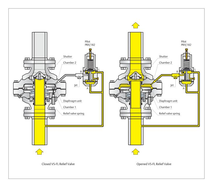
The diaphragm unit (permanently connected to the shutter) divides the relief valve actuator into two chambers.
